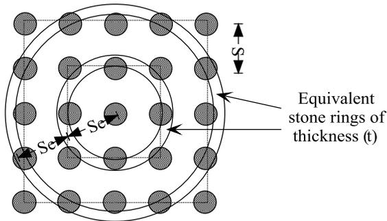
Fig. 1 - Concentric rings idealization for group of 5x5.
