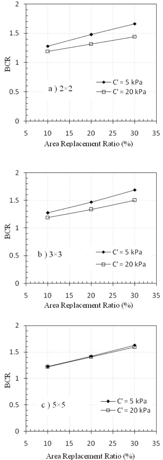
**Fig. 5 - Effect of soil cohesion on BCR**
