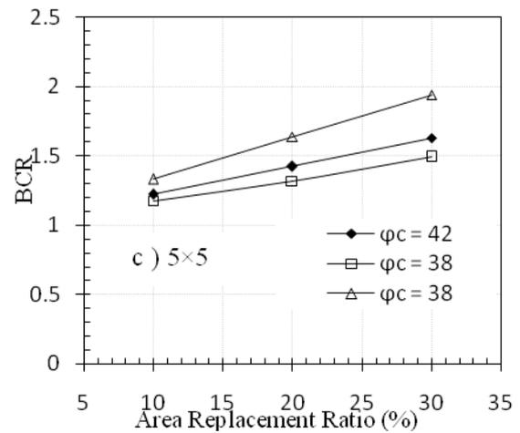
Fig. 7 - Effect of stone column friction angle on BCR
