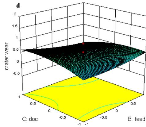
Figure 6: 3-D surface plots a) Interaction effect of feed and speed on the crater wear b) Interaction effect of speed and reinforcement on the crater wear c) Interaction effect of depth of cut and speed on the crater wear and d) Interaction effect of depth of cut and feed on the crater wear.
