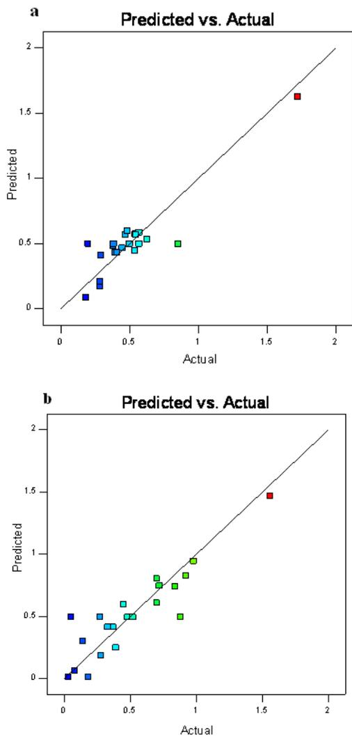
Fig. 3: Relationship between experimental and predicted values (a) Flank wear (b) Crater wear
