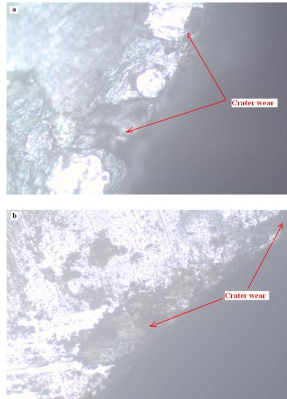
Figure 7: Optical micrograph showing crater wear a) 2 % reinforced b) 8 % reinforced (100X)
