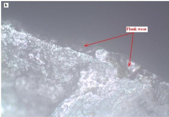
Figure 5: Optical micrograph showing flank wear a) 2 % reinforced b) 8 % reinforced (100X)
