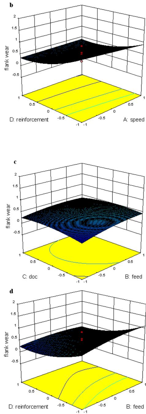
Figure 4: 3-D surface plots a) Interaction effect of feed and speed on the flank wear b) interaction effect of speed and reinforcement on the flank wear c) Interaction effect of depth of cut and feed on the flank wear and d) Interaction effect of reinforcement and feed on the flank wear.
